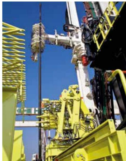
2-stage pipe handling between vertical pipe rack and well center
