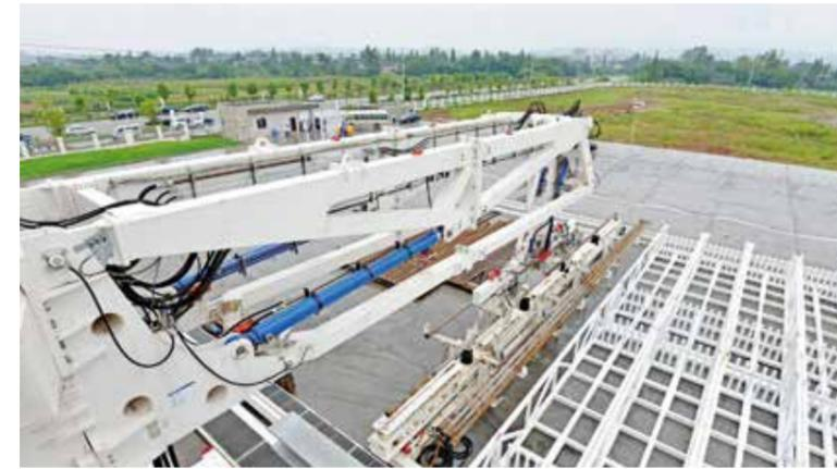
Automated pipe handling and racking system controlled from the driller’s cabin.
