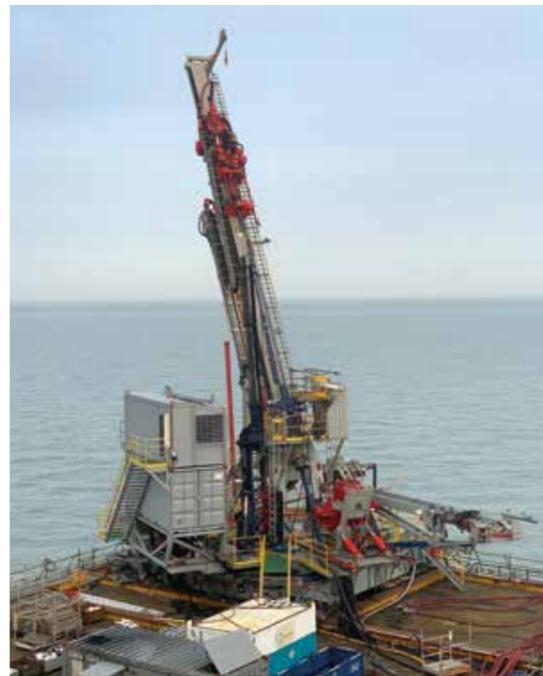
Rig operating in SDD mode on existing slanted well slot
