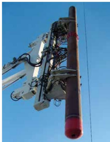
Hands-off pipe handler for safe handling of drill string and casing
