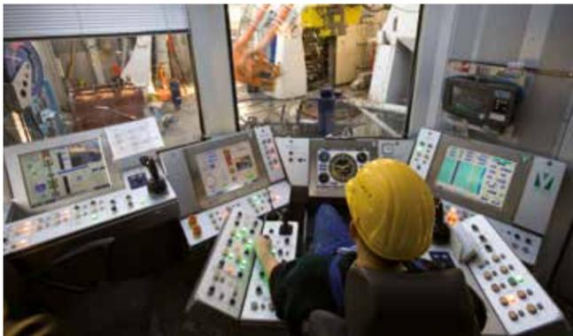
Modern driller's cabin to control rig and pipe handling operations
