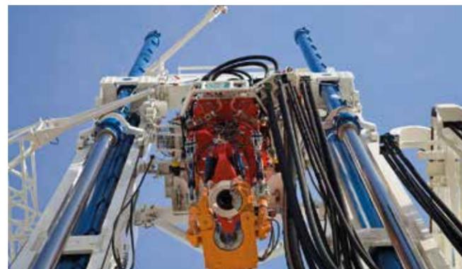
Hydraulic cylinder hoisting system and rotary top drive
