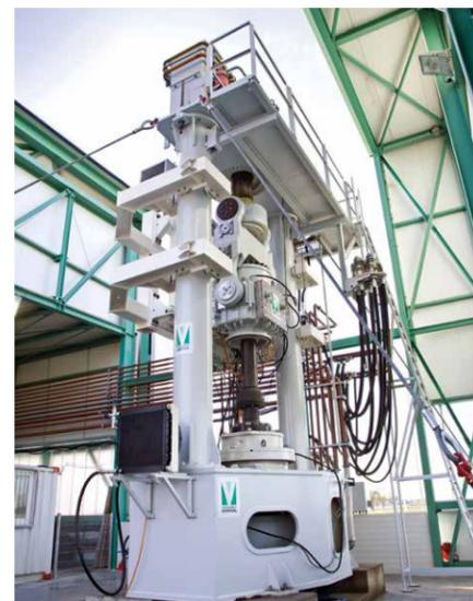
Hydraulic top drive and hoisting dolly at rack & pinion rig
