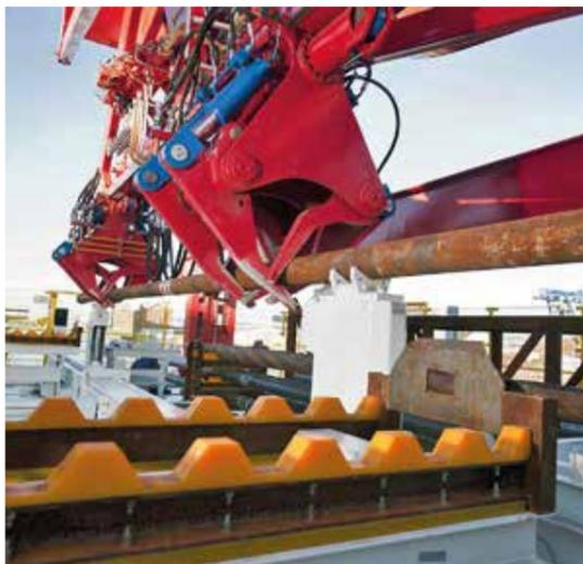
**Pipe handler gripper** and pipe yokes on catwalk
