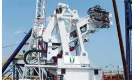
**Herrenknecht Vertical's hydraulic pipe handling modernization package** automates conventional vertical pipe racking in the mast, eliminating the hazardous work of the derrick man and rig floor personnel. Tubulars are handled safely and highly efficient by applying PLC-controlled continuous repetitive movements. The upgrade package works hand in hand with customer's equipment, such as catwalk, iron roughneck elevator and top
