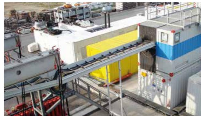
Integrated extension system between rig and backyard for easy and fast skidding without disconnection of hoses and cables
