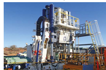
RAISE BORING RIG RBR900VF
