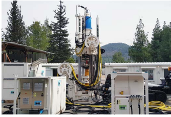
RAISE BORING RIG RBR300VF
