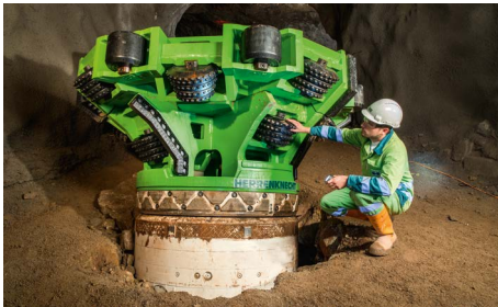
Reaming head on boring unit before collaring.
