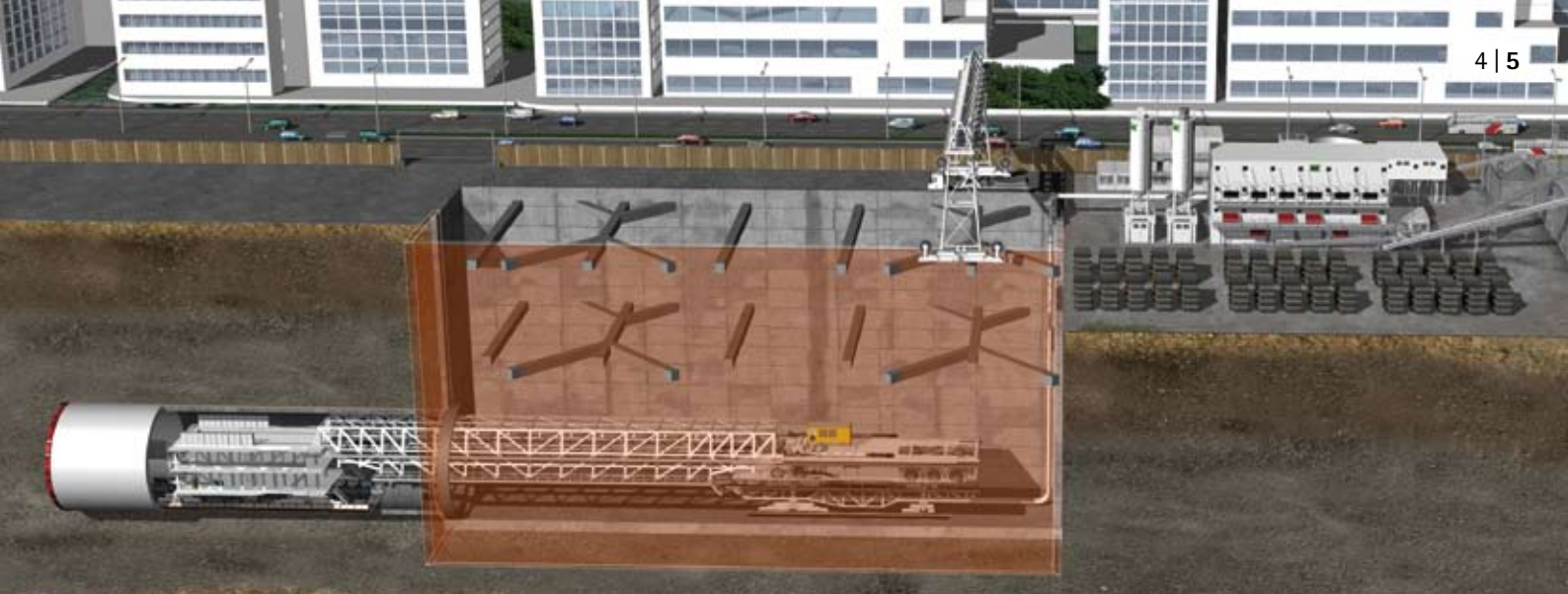
Tunnelling jobsite with Herrenknecht tunnelling machine and separation plant.
