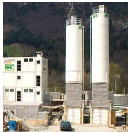
HK60 Herrenknecht bentonite mixing plants with silos.
