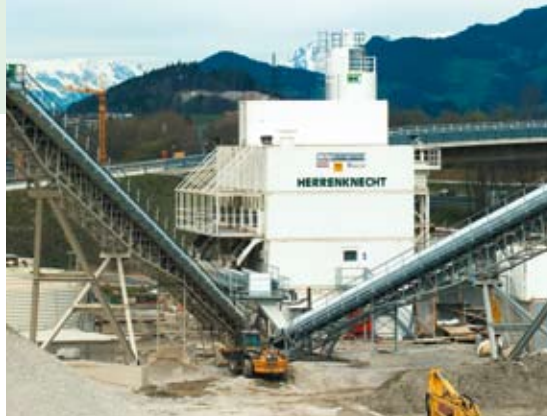
The Herrenknecht HSP2800 separation plant for the Herrenknecht S-381 Mixshield (Ø 13m) in Jenbach, Austria.
