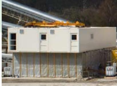
Covered HK84 downstream decanter centrifuges on the H8 tunnelling jobsite in Jenbach, Austria.
